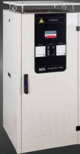
The Protect RCS TPRe TD battery charger system has been developed and designed to provide high reliability power supply and battery charging capability. The Protect RCS TPRe TD is a thyristor-controlled battery charger suitable for charging nickel-cadmium or lead-acid batteries while supplying DC loads. Its design is optimized for T&D (Transmission and Distribution) applications.
