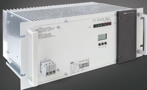
The DC 3000 from AEG Power Solutions is a DC/DC-Converter, converting either 110 VDC or 220 VDC to 24 VAC with an output current of 100 A. The switch-mode power supply is fed by the secure 110 V or 220 VDC supply for high operating reliability.
